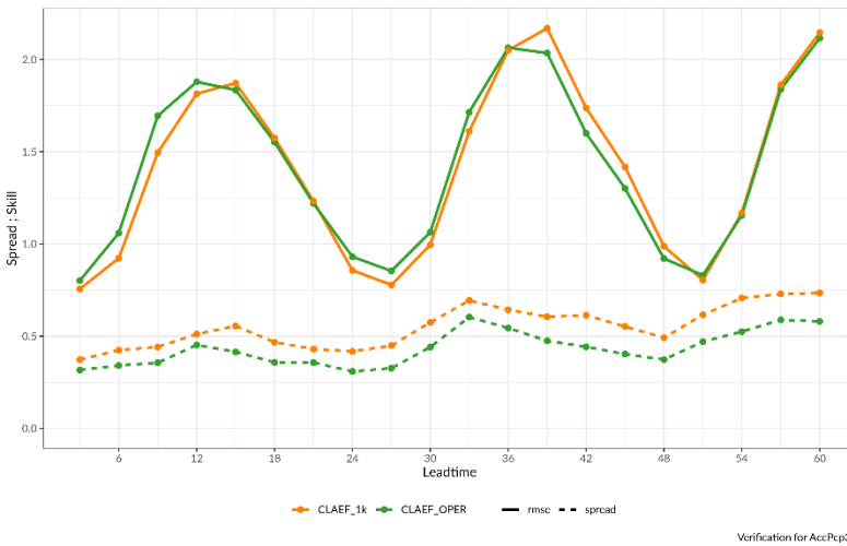
Figure 12: Spread (dashed) and skill (RMSE, full) of 3 h accumulated precipitation (left) and 10 m wind speed for C-LAEF 1k (orange) and C-LAEF operational (green) for a test period in winter 2025.
