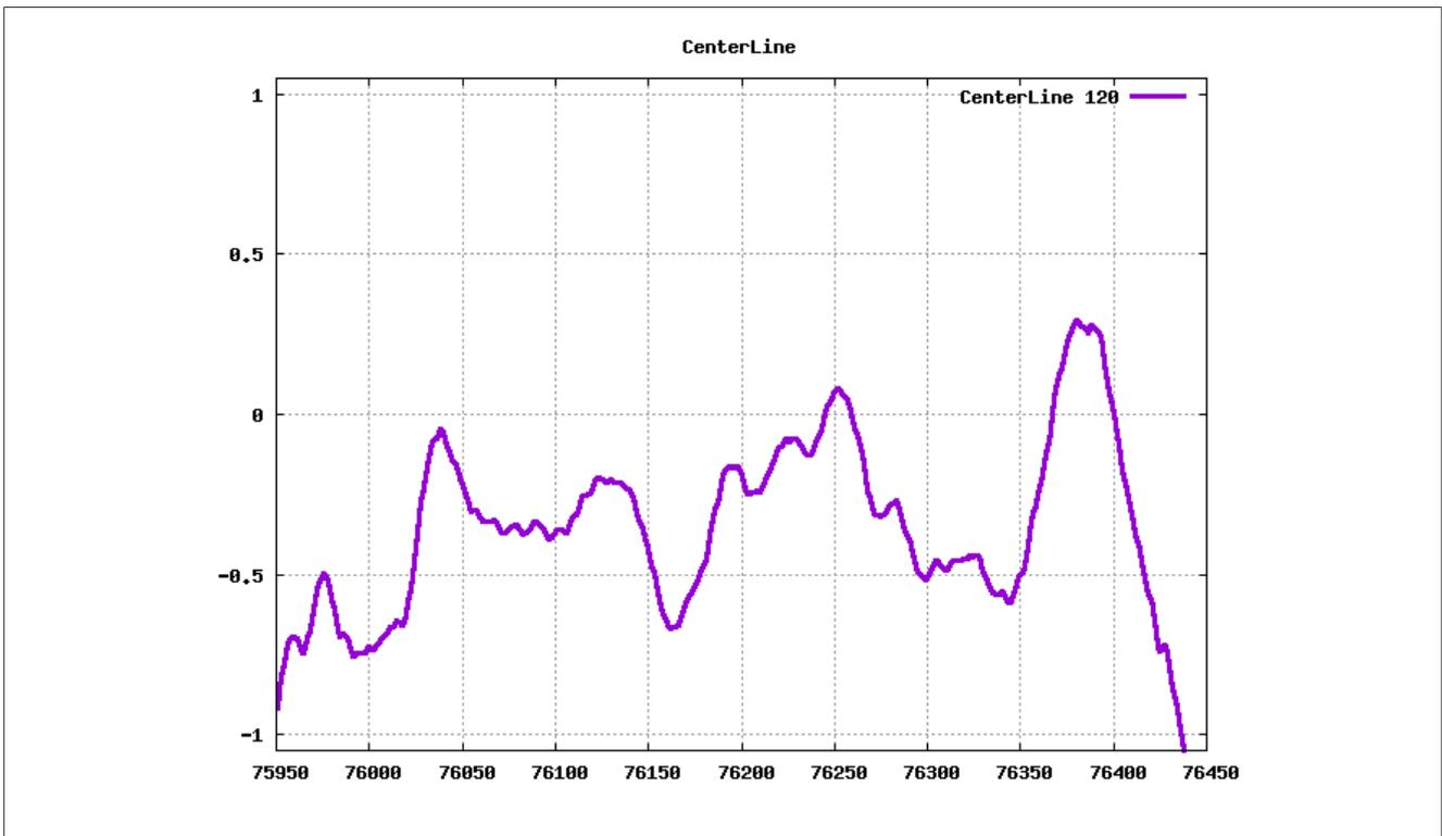
**Fig.3:** An x-oriented cross-section of the random pattern generated by SPG (in ALADIN code implementation).
