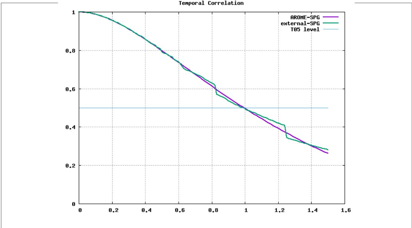
**Fig. 7.:** Temporal correlation functions calculated from fields of ALADIN code implemented SPG fields (purple) and from external SPG program results (green). Blue line shows the 0.5 level.
