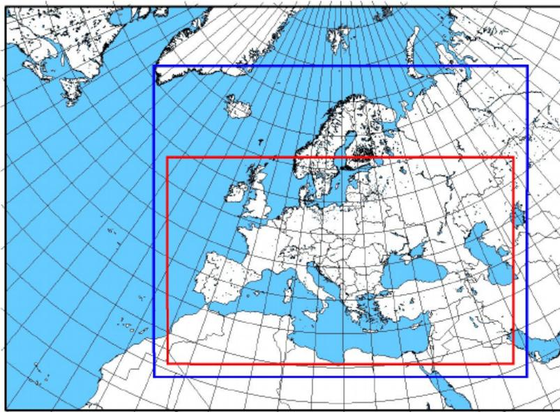
Figure 2: ALADIN-LAEF integration domains: the current one at 11 km horizontal resolution (blue) and the new one at 5 km horizontal resolution (red).
