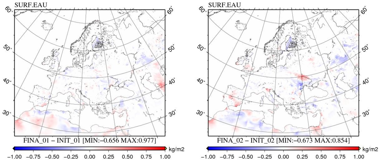
**Fig 9:** Surface liquid water content assimilation increments after revised Relative Humidity assimilation for ensemble member 01 (left) and 02 (right). The differences between the members are due to perturbed observations.
