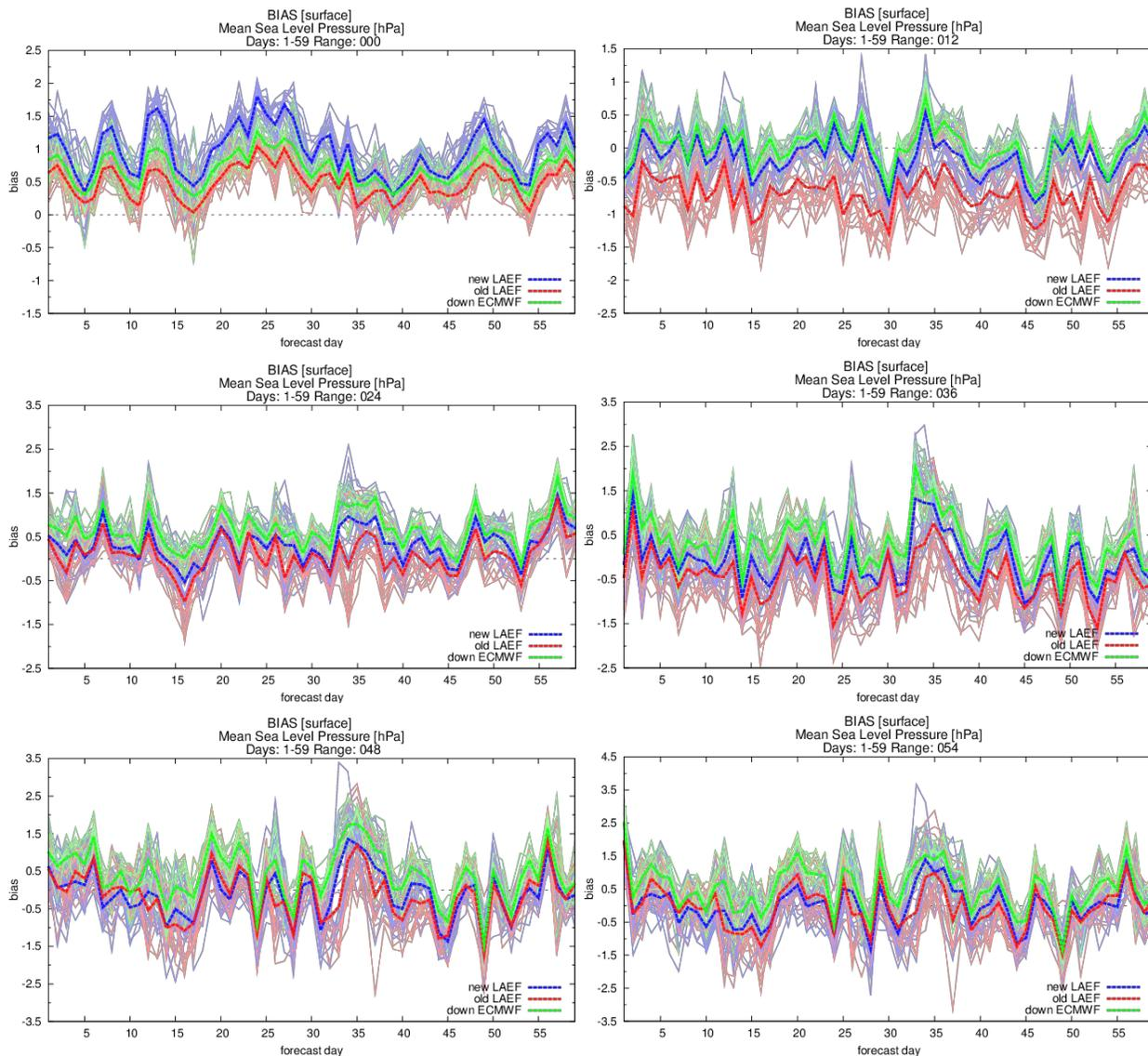
**Fig 18:** Ensemble mean BIAS (bold dashed lines) for MSLP by forecast days and the same for 16 individual ensemble members respectively (thin lines) for range 00, 12, 24, 36, 48 and 54 (ordered from the upper left corner to the bottom right). New LAEF is blue, old LAEF is red and ECMWF downscaling is green.
