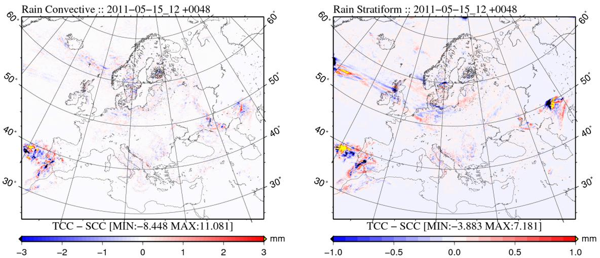
**Fig 5:** The difference between TCC and SCC experiments for accumulated Convective Precipitation (left) and Stratiform Precipitation (right) valid for 17<sup>th</sup> of May 2011, 12 UTC.
