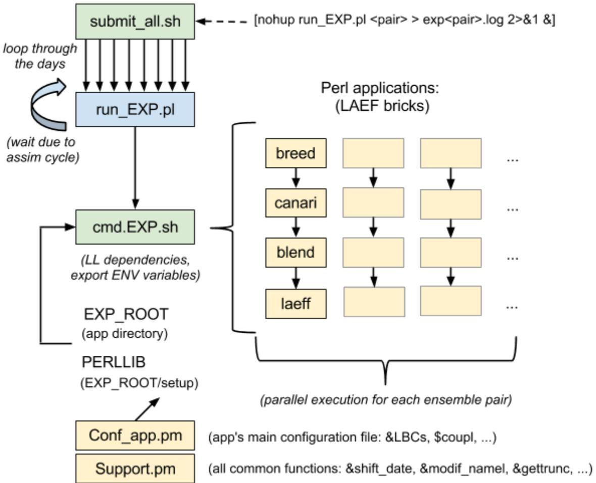
**Fig 10:** New ALADIN-LAEF development scheme used for the experiments (such canari and blend “bricks” are used in the operational ALADIN-LAEF suite as well).
