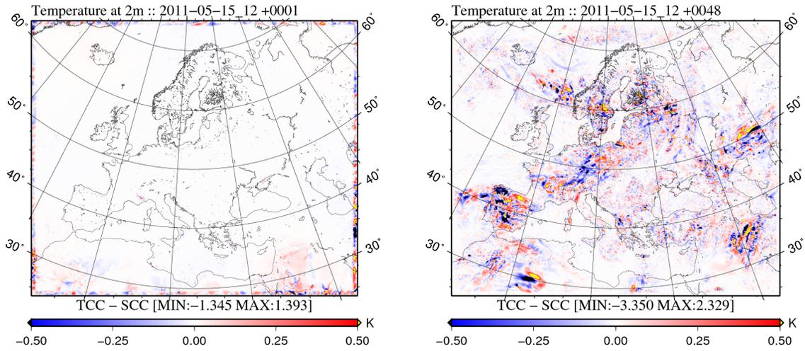
**Fig 2:** The difference between TCC and SCC experiments for Temperature at 2m after 1<sup>st</sup> hour of integration (left) and after 48 hours, i.e. valid for 17<sup>th</sup> of May 2011, 12 UTC (right).
