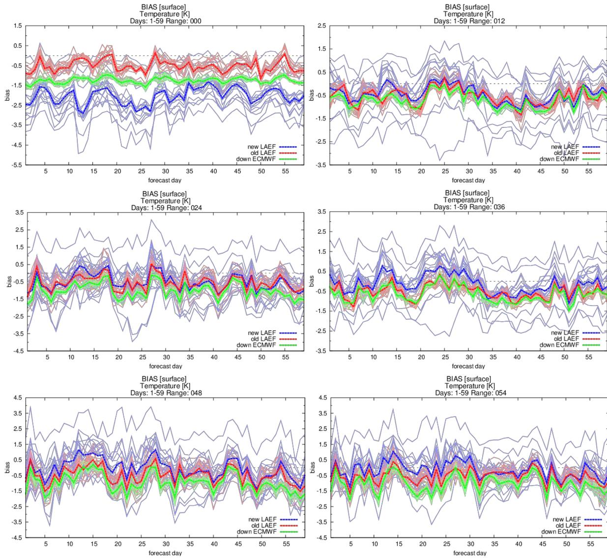
**Fig 17:** Ensemble mean BIAS (bold dashed lines) for the Temperature at 2m by forecast days and the same for 16 individual ensemble members respectively (thin lines) for range 00, 12, 24, 36, 48 and 54 (ordered from the upper left corner to the bottom right). New LAEF is blue, old LAEF is red and ECMWF downscaling is green.
